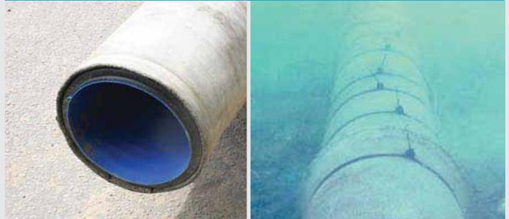
CC can be used as a coating for overland or underwater pipeline protection, providing a superior tough rock shield. In remote areas it can be used to coat steel pipe on site without expensive wet concrete application plants. CC will set underwater and provide negative buoyancy. CC13 meets the requirements of ASTM G13 (Standard Test Method for Impact Resistance of Pipeline Coatings).
