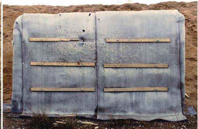
Concrete Cloth reinforced wall after 800 rounds
